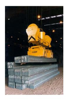
BIPOLAR LIFTING ELECTROMAGNETS FOR LONG PIECES OF HIGH SECTION
